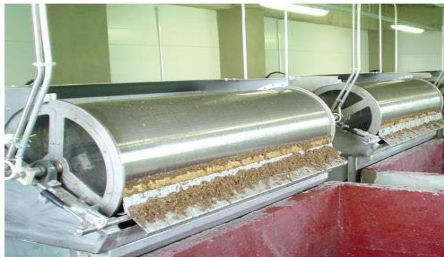
Series of Drum Screens used in brewery industry
